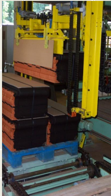
Ziegelhandling Brick Handling
