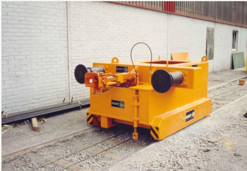
Wagenschubanlage Car Pushing Device
